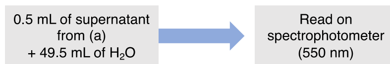
Figure 1. Overview of POXC protocol and the two overall steps of (a) sample reaction and (b) sample dilution.
