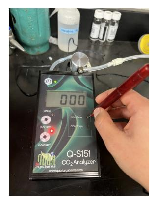
**Note:** If the zero reading is highly out of range (>40 ppm) or if rotating the CO<sub>2</sub> Zero does not work, the Coarse Zero adjustment on the back of the analyzer can be used to bring zero within range. Use the Coarse Zero with caution since very small adjustments result in large changes and there is delay in response to changes in Coarse Zero.
