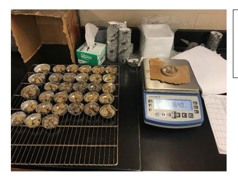
Weighing GWC samples post 24 hour drying period to record Soil + Tin weight after drying. Cardboard is used to protect scale if samples are weighted immediately after removal from oven.
