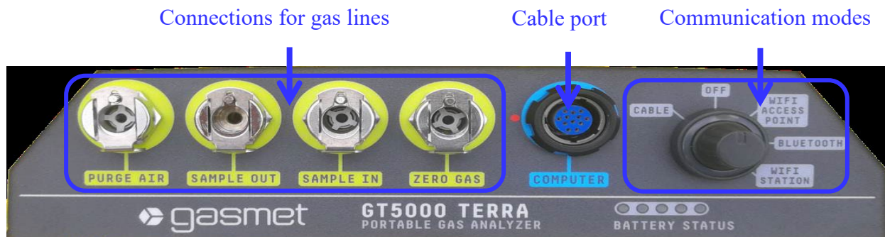
Figure 3. Close-up of Gasmet machine. Connection for gas lines, cable port, and communication modes are circled and labeled. Note latch mechanism on gas lines,
