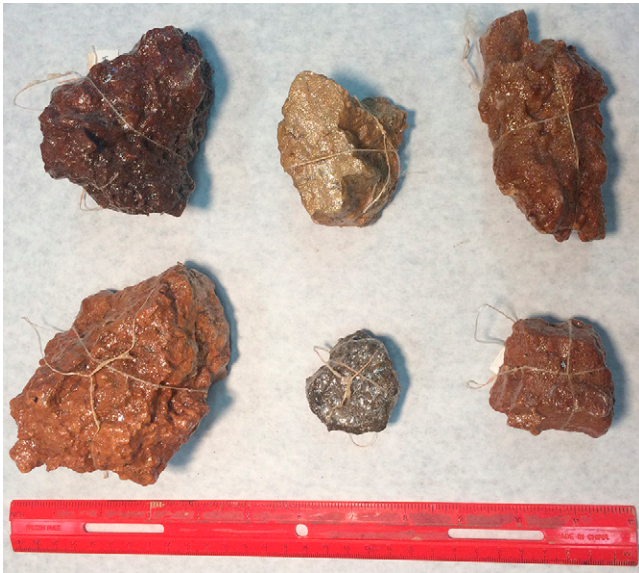
Fig. 2. Paraffin-coated peds used to demonstrate differences in soil structure and color to primary school students. Coating of peds enabled their use, whereas handling of untreated soils (e.g., soil texture by feel) was not possible due to hygiene and cleanliness constraints of the hosting institution.
